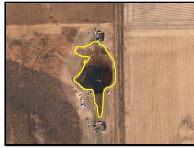
Figure 2. Identification of a Liquid Hydrocarbon Spill with Geospatial Outline of the Affected Area.
